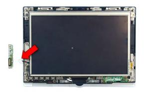
9. Connect the cable to the new Fingerprint Sensor board and place it into the rear cover.
