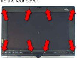
11. Press the front cover into place and secure it with 8 screws.
