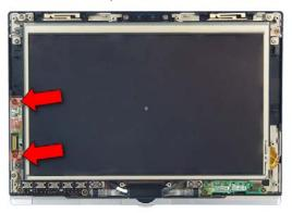
7. Extract 2 screws from the Fingerprint Sensor board.
