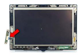
8. Disconnect the cable from the board and lift it out.
