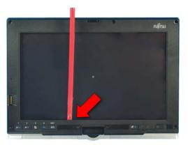
5. Gently slide the pry tool between the screen and the front cover to release the tape.
